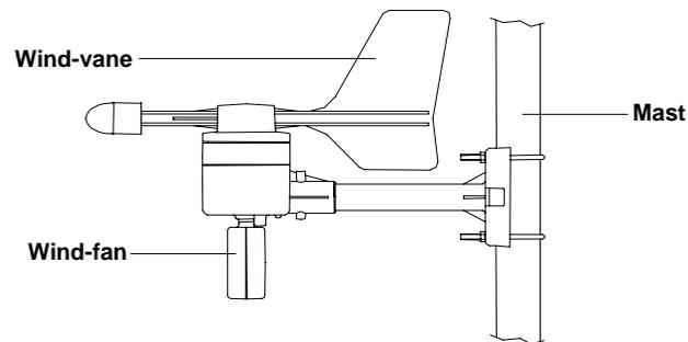
Firstly, check that the wind-fan and the wind-vane can rotate freely before fixing the unit. For correct and accurate readings it is important to mount the sensor so that the front (marked E) is pointing in East-West direction. The wind sensor should now be mounted using the screw provided onto a mast to allow the wind to travel around the sensor unhindered from all directions (ideal mast size should be from  $\varnothing 0.63'' - \varnothing 1.3''$ ).
