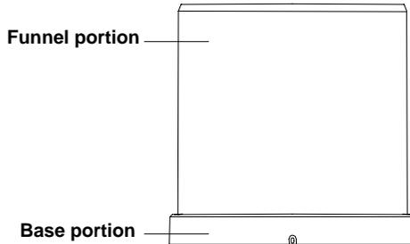
For accurate results, the rain sensor should be securely mounted onto a horizontal surface about 2-3ft above the ground and in an open area away from trees or other coverings where rainfall may be reduced causing inaccurate readings.
