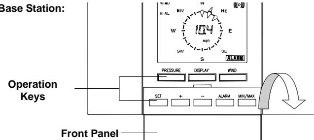
**Note:** flip open the front panel under the PRESSURE, DISPLAY and WIND keys to reveal the SET, + (plus), - (minus), ALARM and MIN/MAX operation keys
