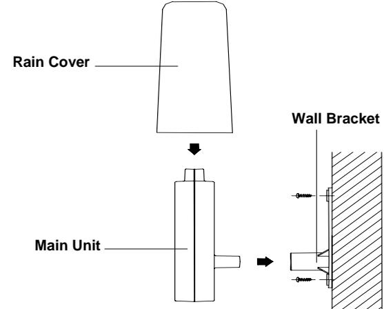
An ideal mounting place for the thermo-hygro sensor would be the outer wall beneath the extension of a roof, as this will protect the sensor from direct sunlight and other extreme weather conditions.
